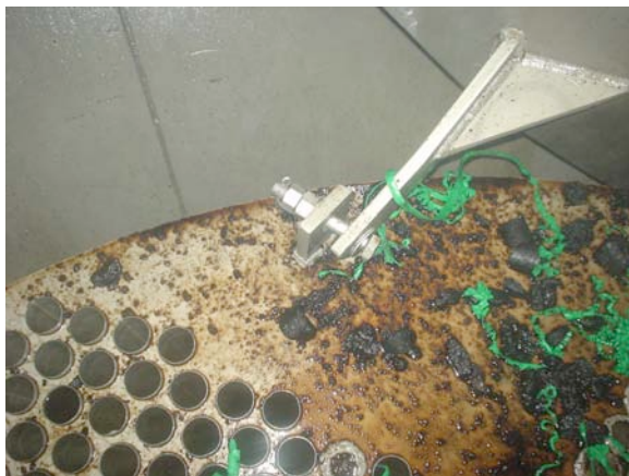
C1 EFFECT LOOSE UMBRELLA HOLD DOWN BOLT
